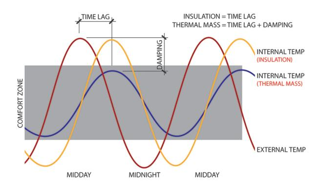
Take a look at this graph to help visualise what ICF is doing. This shows the difference between insulation and thermal mass individually in a cyclic climate. ICF has a even greater effect because it combines both advantages extending the time lag and increasing the dampening effect.
